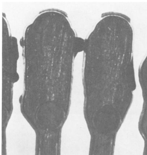
FIG. 5—Circular ejector pin markings visible on rear of backpads. Ejector pins push upward on printwheel to remove it from mold. Note also plastic bridge between the two spokes, caused by warpage of the soft mold under the pressure of the thermoinjection molding process.
